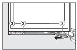
With the three screws ③, first screw on the spacer on the handle side and then the soft-close mechanism on the appliance side.
