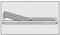
Remove the two active charcoal filters and insert the new filters into the retainer with the encircling edge down.
