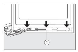
Open the bottom door of the appliance. ■ Loosen the panel ① of the soft-close mechanism: Slowly pry the panel off from the top.
