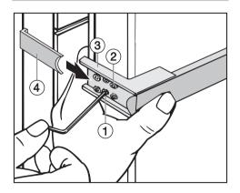
First, loosely screw the door handle onto the opposite side with the two front screws 2. The mounting plate ③ must be positioned on the door housing in such a way that when the door is **closed** the mounting plate is aligned with the outside wall of the appliance. If this alignment is off, you can correct it by
