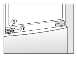
Put the bearing pin (9) in the middle of the appliance through the hinge bracket (11) into the bottom door of the appliance.
