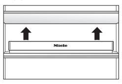
■ Pull the retainer for the active charcoal filters up and off the shelf.
