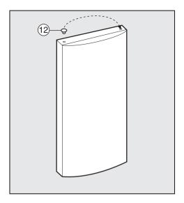
■ Lift the plugs ② out of the door bearing bushing in the appliance door and place it on the other side.
