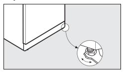
■ Use the wrench provided to adjust the feet as needed, so that the appliance is level.
