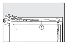
■ Loosen the panel ① from the soft-close mechanism: From below, slide a flathead screwdriver into the recesses, then slowly and carefully lift off the panel.
