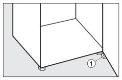
■ If necessary, unscrew the foot ① from the hinge bracket in order to support the appliance door.
