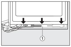
■ Remove panel ① from the soft-close mechanism and ease it off carefully from above bit by bit.
