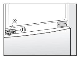
■ Fit hinge pin ⑨ into middle hinge plate ⑪ in the lower door.
