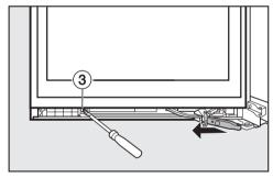
■ Screw the spacer and the soft-close mechanism together securely using screw ③.
