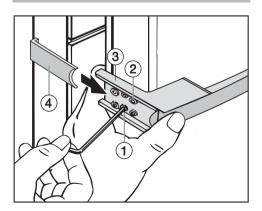
■ Loosely attach the handle to the opposite side of the door with the two front screws ②.
