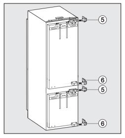
■ For 16 mm cabinetry walls only: Clip the spacers ⑤ and ⑥ onto the upper and lower hinges.
