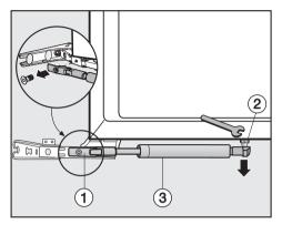
■ Leave the hinges open and remove the screw in the mounting ①.
