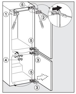
■ Using a flathead screwdriver, lift and remove the covers ①, ② and ③, as well as the plugs ④.
