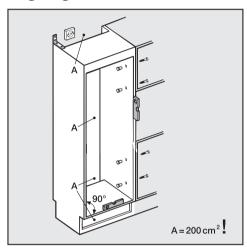
Before installing the appliance, the cabinetry must be carefully aligned using a level. The cabinetry corners must be at 90° angles, otherwise the custom door panels will not be flush with all 4 corners of the cabinetry.
