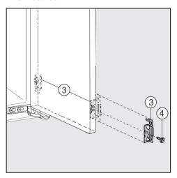
Screw the provided fixing brackets 3 into the pre-drilled holes in the appliance door using a hex screw 4.
