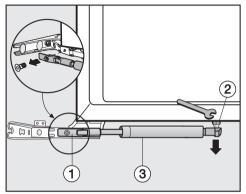
■ Leave the hinges open and remove the screw from the mounting ①.
