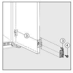
■ Screw the provided fixing brackets ③ into the pre-drilled holes in the appliance door using a hex screw ④.
