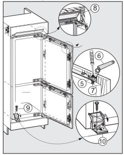
■ While holding the adjusting bolts ⑦ with a screwdriver, tighten the nuts ⑤ on the appliance doors using a wrench ⑥.
