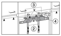
Undo nuts ③ and take fixing bracket
