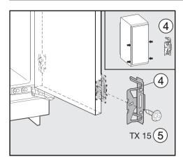
Screw fixing bracket ④ using hex screw ⑤ to the pre-drilled holes in the appliance door.
