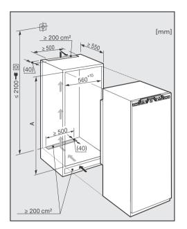
Before installing the appliance make sure the housing unit is the correct size. Specified ventilation gaps must be maintained in order to ensure that the appliance functions correctly.
