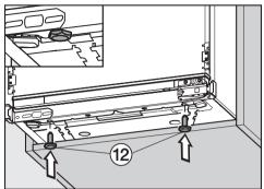
Screw in adjustable feet (2) completely.
