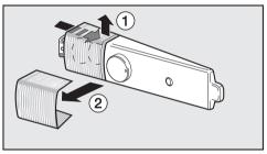
■ Reach into the back of the light cover, press upwards at the side ①, and then pull the cover off ②.
