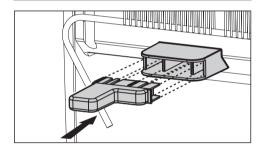
■ Fit the wall spacers onto the back of the appliance on the left and right above the compressor.
