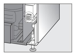
Choose the desired switching contact and connect according to alarm system requirements.
