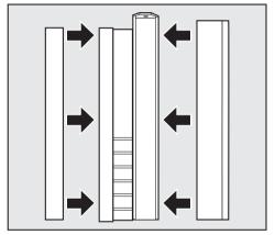
■ If necessary, shorten the three parts of the air separator.
