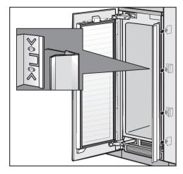
Now attach the covers onto the retaining clips on both sides. In the case of side-by-side installation, the cover strips are only required on the outer side.
