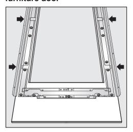
■ Insert the angle trim (5) as far as it will go into the spaces in the frame, as shown.
