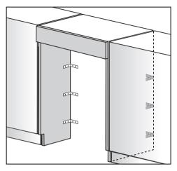
screw the unit to the wall behind using a number of suitable angled fixing brackets. Use suitable wall plugs/fixing screws for the type and material of the wall.
