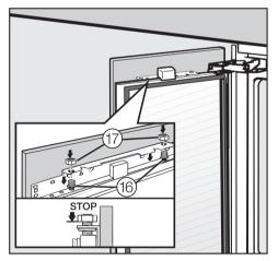
■ Open the appliance door and hang the furniture front on its frame onto the threaded bolts, as shown (16).
