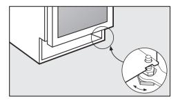
Align the appliance to the height of the niche by altering the adjustable feet using the spanner supplied.
