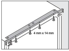
Secure the appliance in its niche by tightening the screws through the fixing strip.
