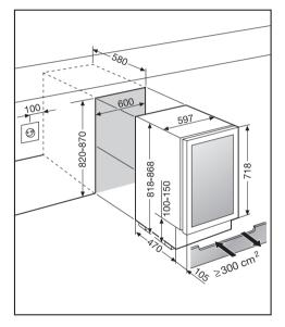
Push the appliance into the niche. When doing this, make sure that the mains cable does not get trapped.
