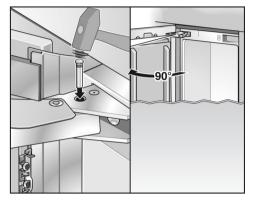
■ Insert the banking pin through the holes and drive in with a hammer.
