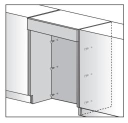
screw the back wall of the cabinet in several places directly to the wall behind it.
