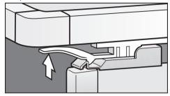
■ On both sides of the drawer, pull the latches (see arrow) upward and lift the drawer out of the refrigerator.
