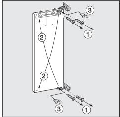
■ Unscrew and remove screws ①.
