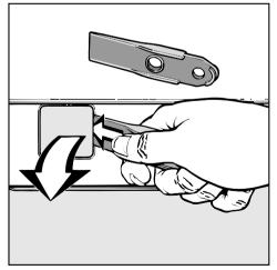
Open the flap (in the machine plinth).
