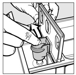
Remove the suction tube from compartment <sup>(a)</sup>, wash under running warm water and put back.
