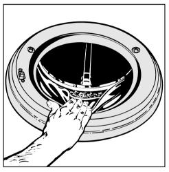
Check the folds in the door seal for any small articles e.g. buttons which might be lodged there. Make sure the drum is empty, items left behind could shrink, or discolour other items in the next wash.
