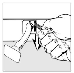
Pull the emergency door latch downwards using a spoon handle (see illustration). The machine door will then open.
