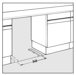
The skids provided with the building under kit \* are intended to prevent damage to floor coverings when manoeuvring the washing machine into position.
