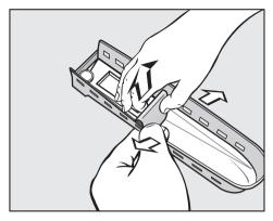
■ Push the insert apart and remove the siphon for easy cleaning.
