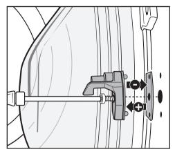
If you use too many spacers the door will not provide a sufficient seal when shut.
