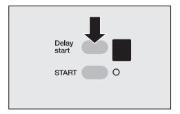
Press the Delay start button repeatedly until the required delay start period shows up in the display (from I to 9 hours).
