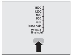
Press the "Spin" button repeatedly until the indicator lamp for the spin speed you want comes on.
