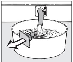
Remove the stopper from the drain hose.
