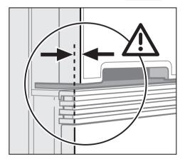
To align the door add or remove the spacers located underneath the door latch.
