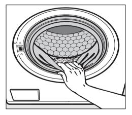
Check the folds in the door seal for any small articles, e.g. buttons.
