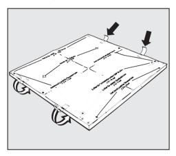
Fix the template in position using adhesive tape.
