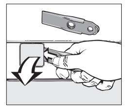
Open the emergency drainage and door release flap in the machine plinth. A Caution: If laundry has been washed at a high temperature, water draining out of the machine will still be hot. Danger of scalding!
