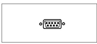
A serial interface is located at the rear of the washer to connect the machine to a PC (Personal Computer).
