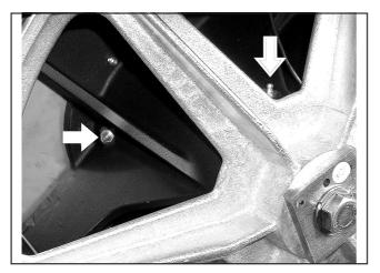
After about 1000 operating hours, lubricate the drum journal bearings with the lubricating nipple using Arcanol L 100 grease.
