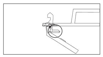
The door handle has lost its function. The door cannot be opened or closed.
