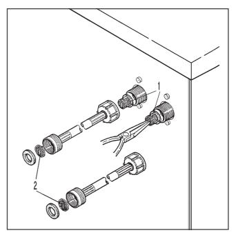
Regularly check and clean the filters in the water intake valves, 1, and the water intake hoses, 2.
