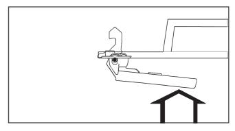
Firmly press against the door handle until you hear the safety mechanism click.
