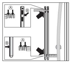
■ Fasten the shipping struts to the rear of the washer. Take care to insert the drill holes correctly, (B), into the clamps, (A).
