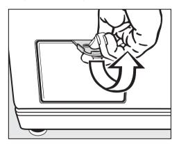
Drain the water from the washer as described in "Cleaning and Care -Cleaning the drain pump and lint trap". Make sure the machine is turned off and the drum has stopped moving. A moving drum is dangerous.
