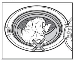
To prevent damage to the door seal and clothing, make sure that there is nothing caught between the drum door and the seal.
