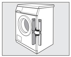
Failure to level the machine can result in increased water and energy consumption, loud noises during the spin cycle or "walking" across the floor during use.
