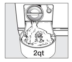
Turn the lint trap lid counterclockwise. Do not remove it. About 2 quarts (2 liters) of water will drain out of the hose.
