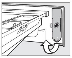
To clean the lint trap, remove the tool from behind the detergent dispenser drawer.
