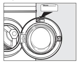
Both can be found on the data plate visible above the front glass on the inside of the door.
