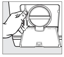
Pull the emergency release cord downwards until the machine outer lid opens.
