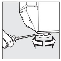
Tighten the counternut using a screwdriver as indicated.
