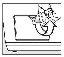
Use the (yellow) filter flap opener supplied with the machine to open the access flap. Place a dish under the drain spout.
