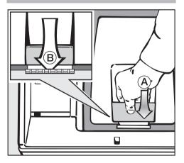
Before closing the inner lid, pull up the lock (A) and engage properly (B).
