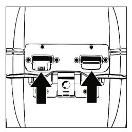
First press the front, then the rear drum flap down until **both** hooks clearly engage.
