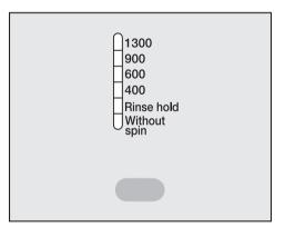
Press the "Spin" button repeatedly until the indicator light for the spin speed you want comes on. In some programmes the maximum spin speed is limited. The machine will not allow a higher spin speed to be selected.
