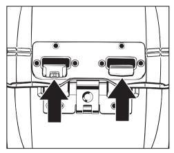
■ First press the front, then the rear drum flap until **both** hooks clearly engage.
