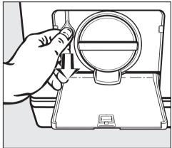
Pull the emergency release downwards until the machine outer lid opens.
