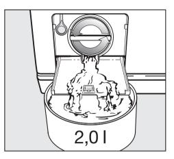
Unscrew the fluff filter lid until water runs out.
