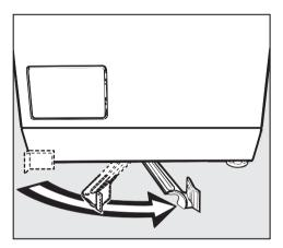
Before moving the machine, swing the transport base lever over to the right.
