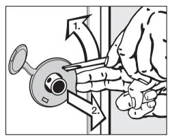
■ Remove the left and right rotary protectors. Unhook, 1, the rotary protectors with a screw driver and remove, 2.
