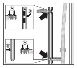
■ Fasten the shipping struts to the rear of the washer. Take care to insert the drill holes correctly, <sup>®</sup>, into the clamps, <sup>®</sup>.
