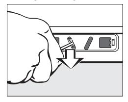
Insert a screwdriver into the notch of the left opening and pull downwards.
