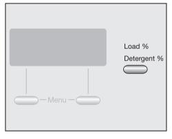
Press and hold the Load/Detergent button pressed in until the following message appears in the display:
