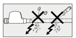
The protective sleeve of the hose must not be damaged or kinked.
