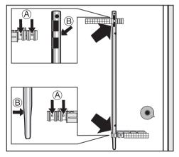
Secure the transit bars to the back of the washing machine. Make sure that holes
