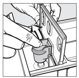
Remove the siphon tube from compartment <sup>(A)</sup>.
