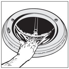
Check the folds in the door seal for any small articles e.g. buttons which might be lodged there.
