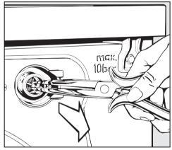
■ Use water pump pliers to withdraw the plastic filter by the bar (see illustration). Clean, put back and secure.
