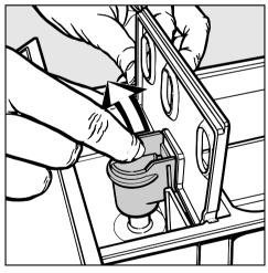
■ Remove the suction tube from compartment , wash under running warm water and put back.
