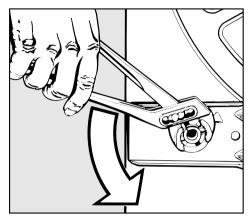
■ Using a pipe wrench turn the lefthand transit bar 90°.
