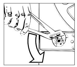
Using a pipe wrench turn the lefthand transit bar 90°clockwise.
