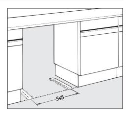
The slides supplied should be used to protect the floor from damage when the machine is pushed into position or taken out for servicing.
