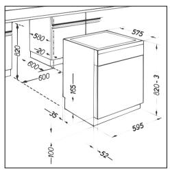
If it is being installed under a 900/910 mm high worktop a raising kit\* is required.
