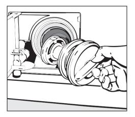
Once the flow of water ceases, remove the fluff filter completely.
