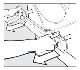
3 Withdraw the two bars together with the support plate.
