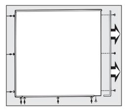
Unscrew the remaining 7 screws from the lower and side decor strips until the decor panel bows slightly. It can then be taken off and a new one fitted.
