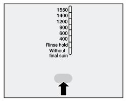
Press the "Spin" button enough times until the indicator light for the required end spin speed lights up.
