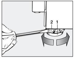
■ Hold the foot **1** firm using a pipe wrench and turn the counternut **2** to the right firmly up against the housing with a screwdriver.
