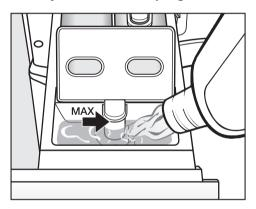
Add the fabric conditioner or liquid starch to compartment \mathscr{R}. Do not exceed the maximum level mark.
