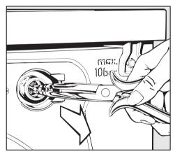
Using needle nose pliers, remove the plastic filter by pulling on the bar (see illustration). Rinse under water and return parts.
