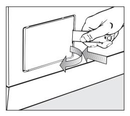
Place a 2 quart capacity container underneath the drain tube.
