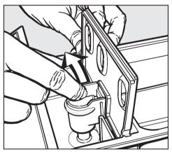
Remove the siphon tube from the fabric softener compartment & and rinse under warm water.
