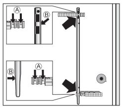
Secure the transit bars to the back of the washing machine. Make sure that holes (a) are fitted over retainers (A). The washing machine must not be moved without the transit bars in place.
