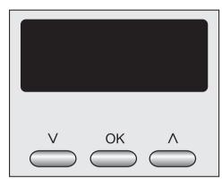
The display is operated using the  $\lor$ , **OK** and  $\land$  buttons.
