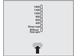
Press the "Spin" button enough times until the indicator light for the required final spin speed lights up.
