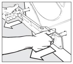
Withdraw the two bars together with the support plate.
