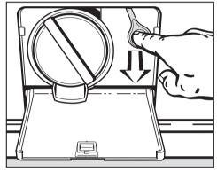
■ Pull the emergency release downwards (see illustration). The drum door will open.
