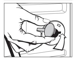
■ Fit the covers on to the two holes. Then plug the holes as shown with the caps.
