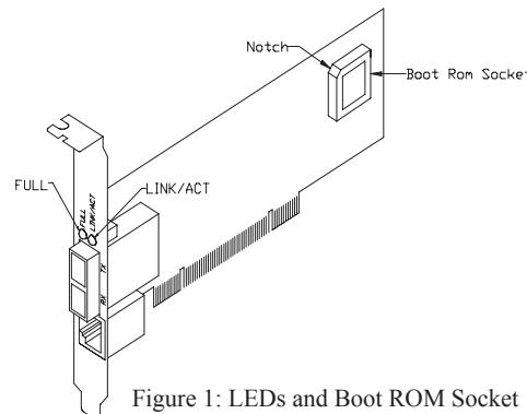
Figure 1: LEDs and Boot ROM Socket
