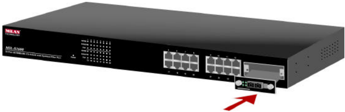
Figure 3-7. Install the 100Base-FX Module by inserting it into the guides and sliding it in until it stops
