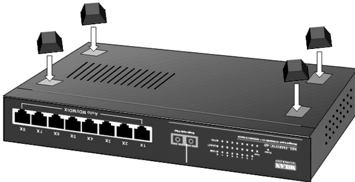
Figure 2-9. Attaching rubber feet to the bottom of the switch
