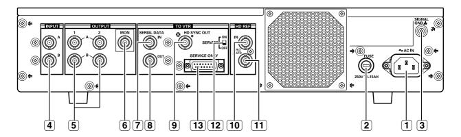
1 AC Input Socket Use the accessory power cord to connect the socket to the power outlet
