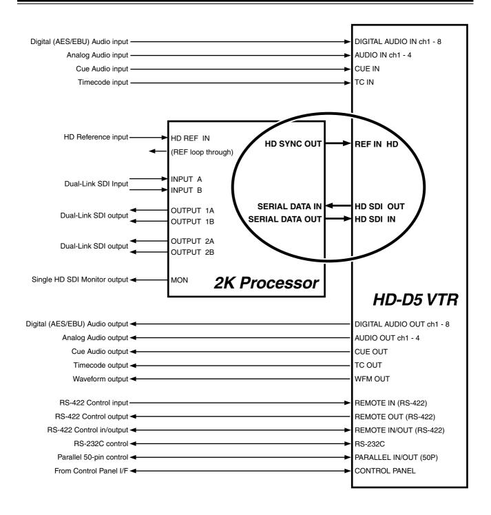
Note: Be Sure to Connect Three I/Os for 2K Processor Systems as below
