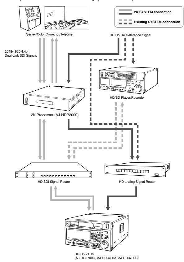
To switch to the 2K system mode, select "2048 (PsF)" or "1920 (PsF)" in F3 (VIDEO) in SYSTEM SET UP menu on the HD-D5 VTR.
