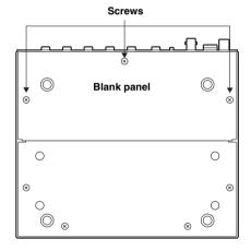
2. Remove the three screws from the rear panel and remove the rear panel.
