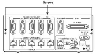
Use the three screws to firmly secure the rear panel where the blank panel was removed from the bottom panel.
