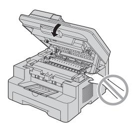
To replace the toner cartridge and the drum unit When the display shows the following, replace the toner cartridge.
