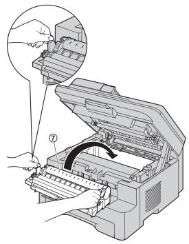
• Make sure that the triangles ((3)) match, to install the drum and toner unit correctly.
