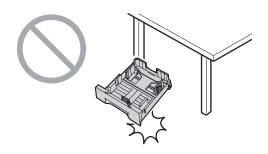
• Hold the paper input tray with both hands when removing or installing. The paper input tray weighs approximately 2 kg (4.4 lb.) when the recording paper is fully installed.
