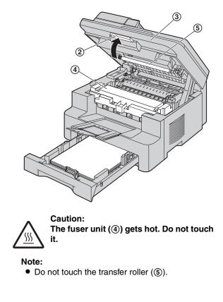
**3.** Remove the jammed paper (**(6**) carefully by pulling it upwards.
