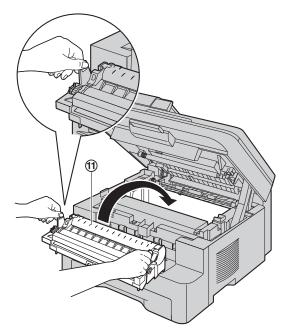
• Make sure that the triangles (12) match, to install the drum and toner unit correctly.
