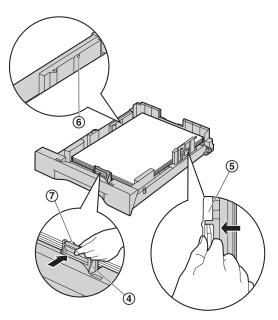
5 Insert the paper input tray to the unit, lifting the front part of the tray. Then push it completely into the unit.
