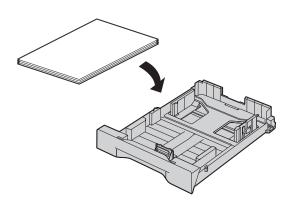
3 Insert the paper input tray to the unit, lifting the front part of the tray. Then push it completely into the unit.
