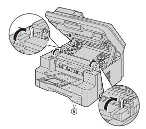
**3.** Remove the jammed paper (⑥) carefully by pulling it upwards.
