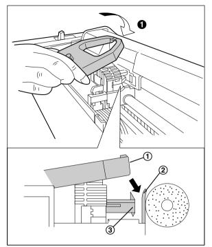
Press down on rear of the ribbon cassette until the wing tab (①) snaps into place.
