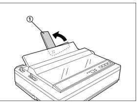
5. Insert a sheet of paper with the printed side face down behind the platen by aligning its left edge
