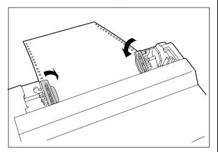
7. Adjust the tractors to remove any slack.2 Lock the tractor clamping levers.
