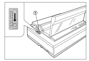
3. Rotate the knob (①) on the ribbon cassette to remove any slack.
