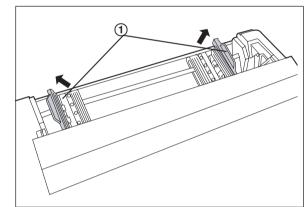
6. Place the paper with the printed side face down and align the paper sprocket holes with the tractor pins, then close the tractor covers.
