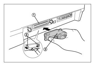
When connecting with a serial interface cable:
