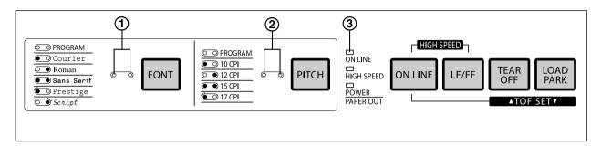
(1) FONT indicators: (2) PITCH indicators: (3) ON LINE indicator: Press FONT. Press PITCH. Press ON LINE.
