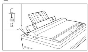
5. Press **LOAD/PARK** to reload the fanfold paper to the first print line.
