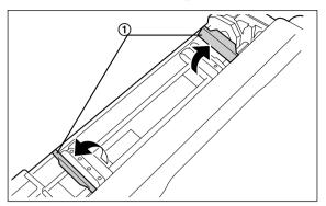
6. Place the paper with the printed side face down and align the paper sprocket holes (②) with the tractor pins (③), then close the tractor cover (①).
