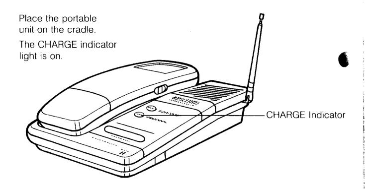
You can use the unit before 10 hours are up. But be sure to put the portable unit on the cradle so it can continue charging.
