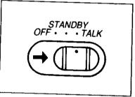
Set to the function selector the "TALK" position to speak the base unit user. The TALK indicator light changes from flashing to a steady light, and the Intercom call is automatically established.
