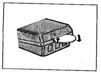
Remove the battery compartment cover using an object such as a coin.
