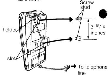
To temporarily place the handset down during a conversation, hook as shown.
