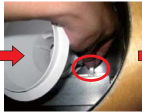
Unplug light unit assembly connector, Then take out the whole assembly
