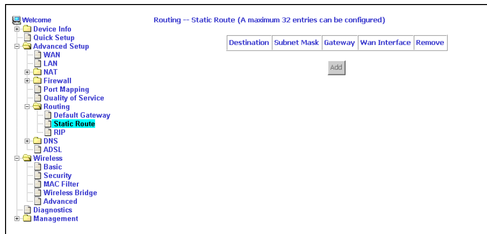
Figure 5-33. Static Route Setup
