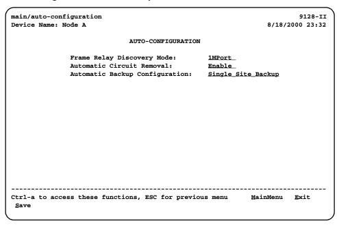
This feature also maintains associated DLCI option settings when Standard LMI is used on the network interface.
