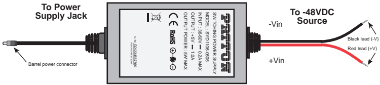
Figure 10. Connecting DC power to the 2707/I DC power supply
