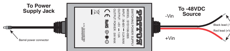
Figure 8. Connecting DC Power to the 2884 DC Power Supply
