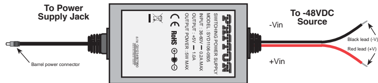
Figure 18. DC Power Supply
