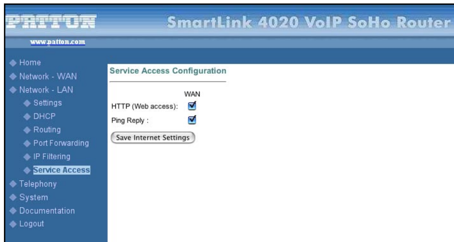
Figure 21. Service Access window
