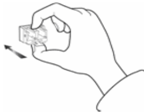
Figure 20 -- Insertion of an Actuator/Button SFP Module
